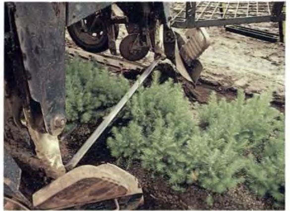
Plate 16. Undercutting. View showing at far end of bed from left to right: i) depth control wheel, ii) vertical coulter cutting track for iii) small disc loosening soil ahead of vertical reciprocating arm carrying undercutting blade. (39556)
