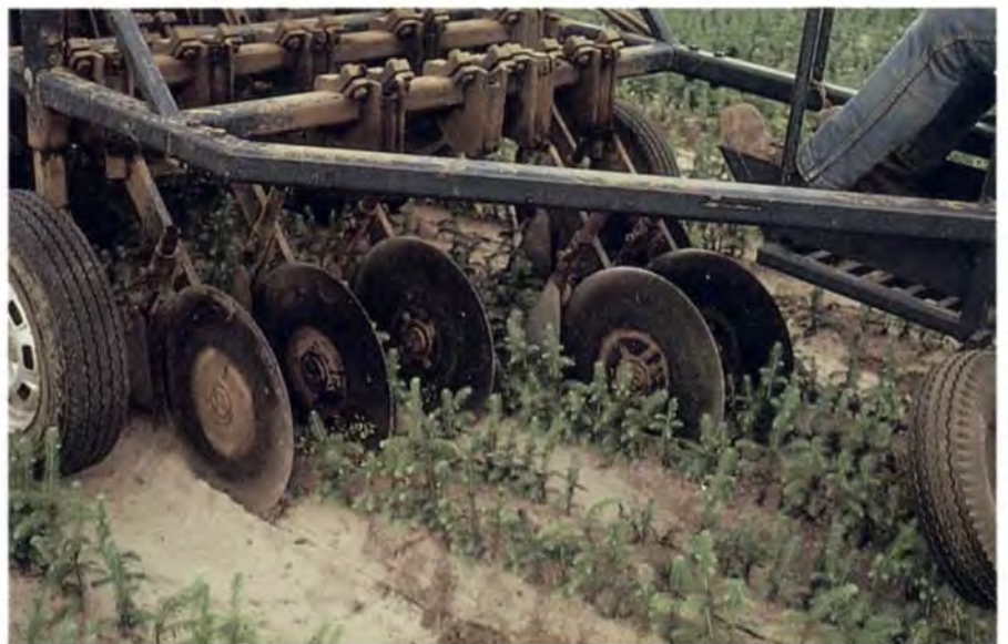
Plate 17. Vertical discs cutting laterals between drilled seedlings. Position of discs controlled by steersman seated on tool-frame. (39550)
