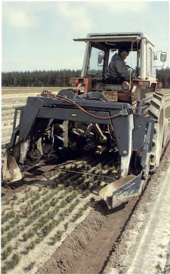
Plate 15. Undercutting. View from rear showing undercutter out of the ground with vertical reciprocating arms and trough shaped shares to restore the edges of seedbeds after the disruption by the reciprocating arms. (E8272)
