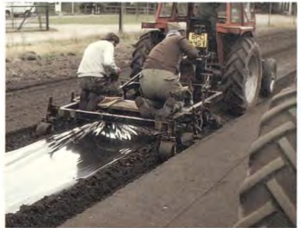
Plate 2. Soil sterilisation using Dazomet. Polythene sheet seal being spread; edges are covered by soil, turned over by small shares one in each alley. (A3184)
