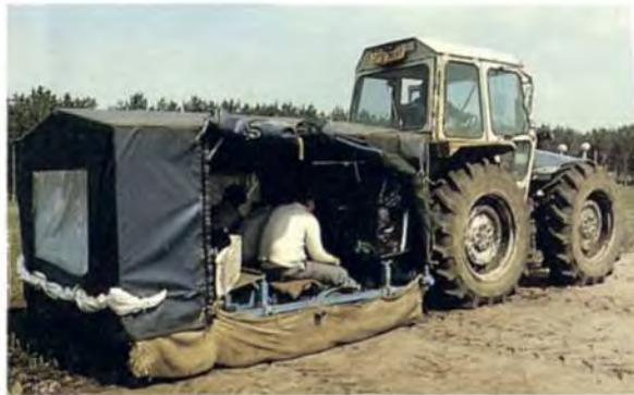
Plate 11. Transplanting using Super-prefer. A general view showing shelter for workers against wind and cold. (E8833)
