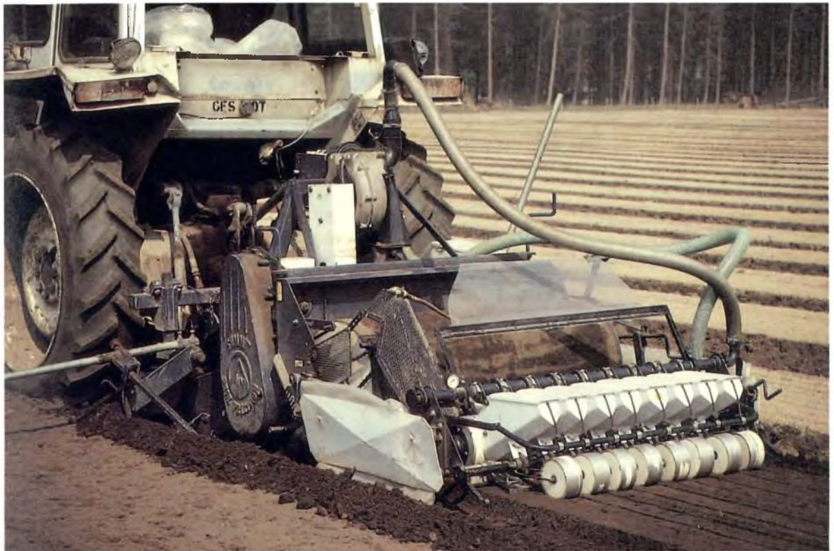
Plate 13. Precision drill sowing by Summit sower, showing: i) vacuum pump on tool frame immediately behind tractor, ii) smoothing roller,
