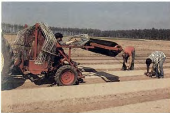
Plate 8. Seedbed being covered with polythene netting against birds showing: i) hoops to hold netting above bed, man feeding them out, ii) netting roll on rotating spindle, iii) netting edges being secured (with pegs). (39386)
