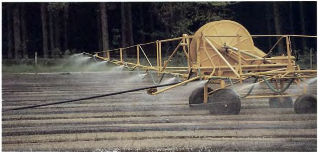
Plate 30. Briggs rainomatic irrigation equipment, showing self-winding hose and reel on carriage. (A1986)
