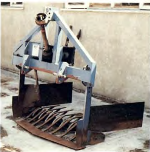
Plate 34. Multi-row plant lifter with secondary vibrating tines to loosen soil. (J.R. Aldhous)
